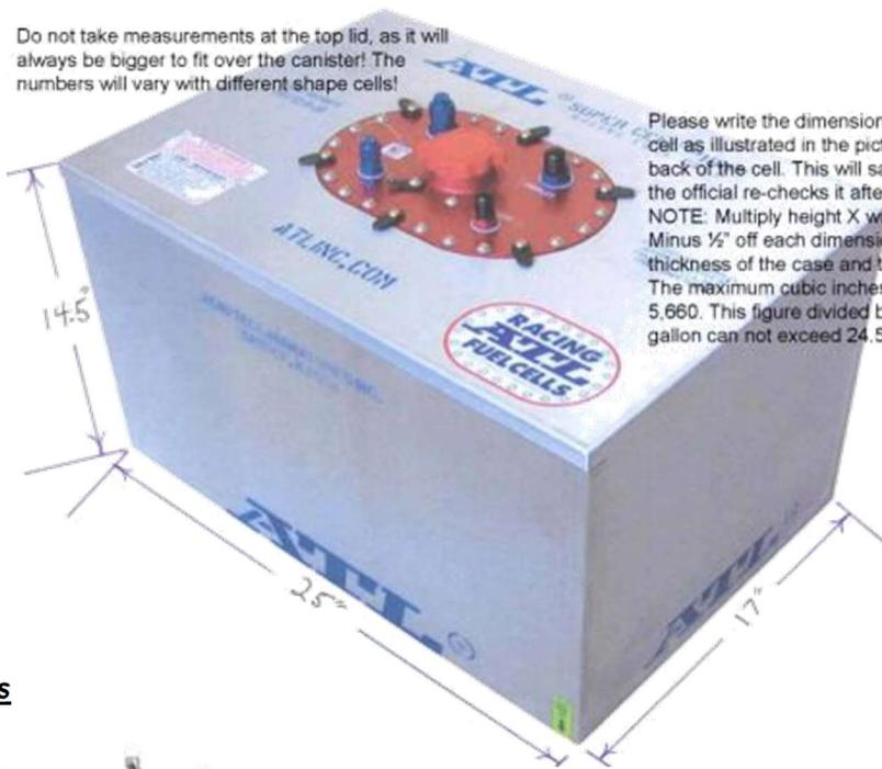
Please write the dimensions of your fuel cell as illustrated in the picture on the back of the cell. This will save time when the official re-checks it after the race. NOTE: Multiply height X width X length. Minus 1/2" off each dimension for the thickness of the case and the bladder. The maximum cubic inches allowed is 5,660. This figure divided by 231 c.i. per gallon can not exceed 24.5 Gallons!!
